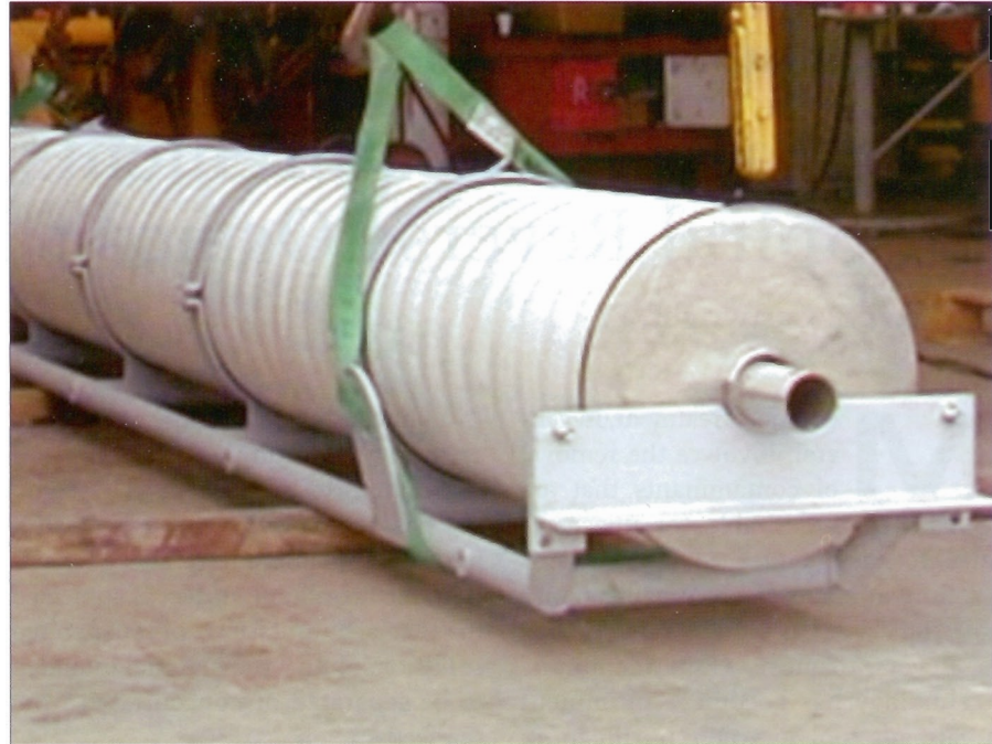
30-inch pipeline in the Gulf of Mexico with 20.0 OD filter
