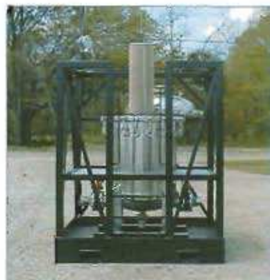
Figure 8. Skid mounted jet fuel filter, 36 in. diameter.
